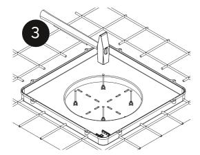
Fix the lower part of the box in place with 4x nails. (Take care that the nail head rests on the plastic dome)
