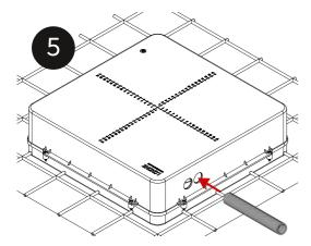
Connect the cable conduit. (Take care to avoid large gaps between back box and conduit)
