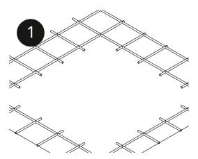
Determine desired location on the concrete formwork and cut out the steel reinforcement
