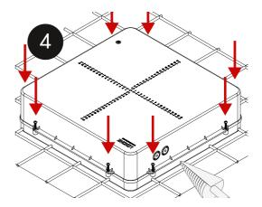
Attach the upper part of the box with the 8x screws. Use a step drill to cut out the holes for the cable conduit
